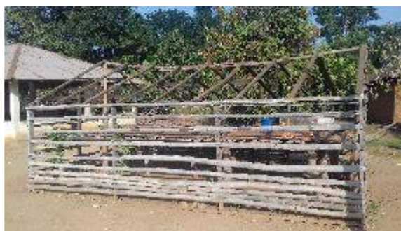
Solar Dryer frame with cover removed.
